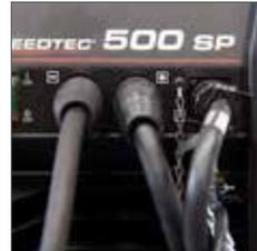
Cable connections on front (standard) and back rear side (an option). All cable connections can easily be made without tools
