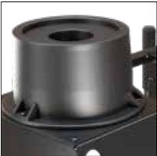
Rotatable wire feeder swivel on the cart enabling rotation of the wire feeder and setting it in any position
