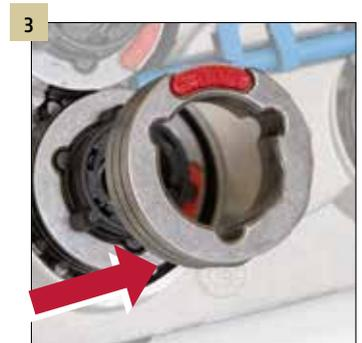
Individually adjustable contact pressure for the front and rear roll pair. Differently set-up for aluminium, steel, stainless steel, braze, flux cored wire
